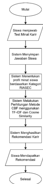
Gambar 5. Diagram Alur Sistem
