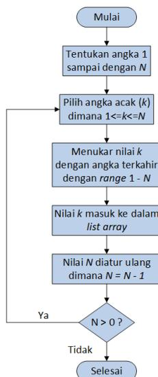
Gambar 5. *Flowchart* Algoritma *Fisher Yates*
