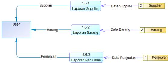
Gambar 5. DFD Level 2 Proses Laporan
