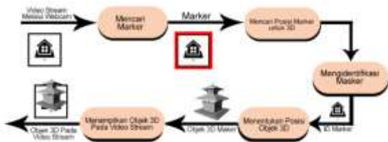
Gambar 2.1 Kerangka Kerja Augmented Reality
